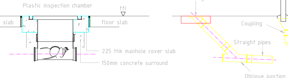
TYPICAL DRAINAGE DETAILS 1:30
